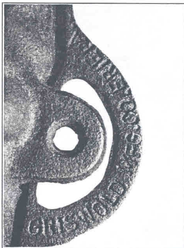
Figure 4: Lettering on the repro are uneven and poorly aligned.
