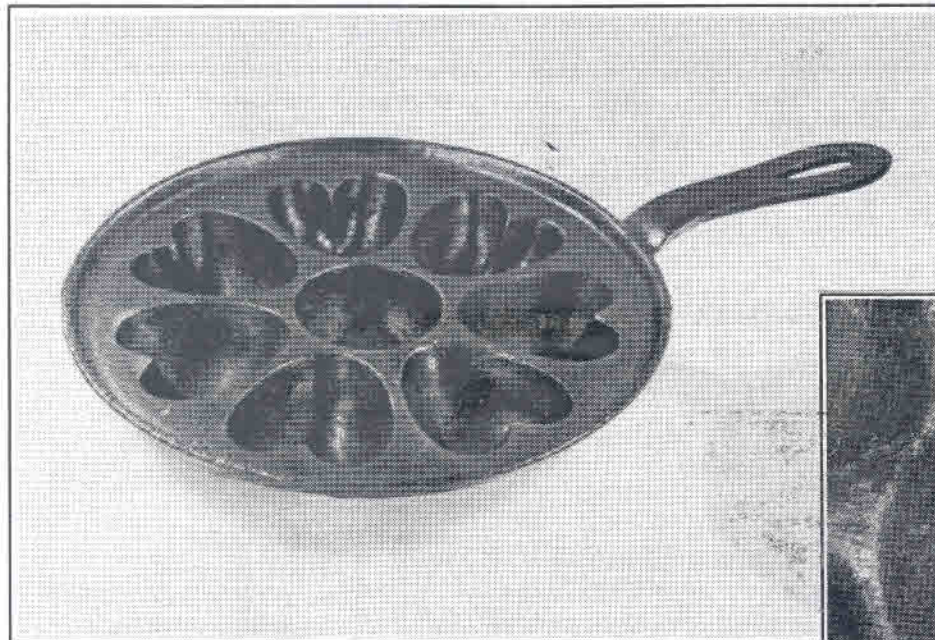
Figure 3: Early 19th century Heart Pattern. Note the sprue mark on the bottom (inset). This was an early casting method. The sprue is the entry point of the molten iron into the mold. Diameter 9", Handle 5", Cups 1" deep. Hearts are rounded verses pointed in Fig. 2.
