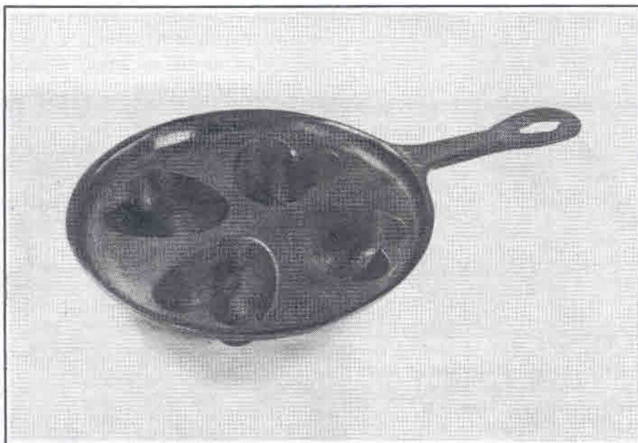
Figure 5: A very unusual four section pattern. It appears to have been cast from the top which is very unusual, and the sprue polished off. Diameter 7 1/2", Handle 4 1/2", Cups 1" deep
