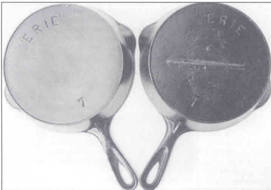
fig. 6 - Comparison of a "New Series" ERIE No. 7 skillet; and a skillet with gate mark that was cast from a pattern made from a "New Series" ERIE No. 7 skillet. Note the difference in the quality of the two castings.
