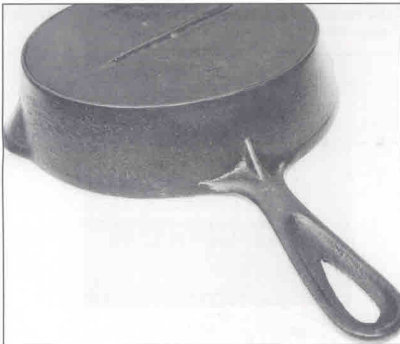
fig. 7a (top photo) & 7b - "New Series" ERIE skillet [fig. 7a] is much better quality than ERIE skillet with gate mark [fig. 7b].
