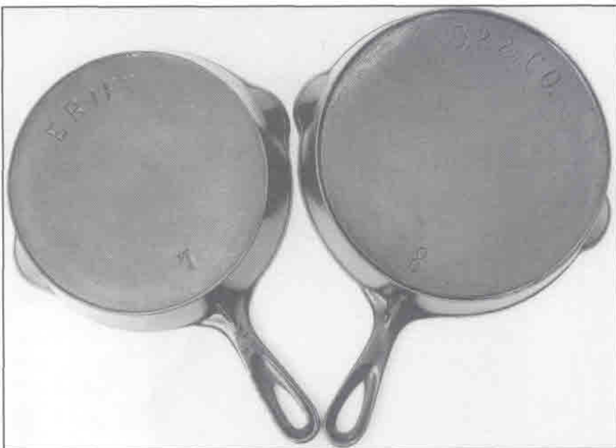
fig. 9 - Orr, Painter & Company skillets (right) were based on the "New Series" design ERIE (left), both the handle and pouring lips.
