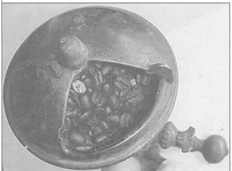
Fig. 4 Sliding cast dome houses coffee beans to be ground
