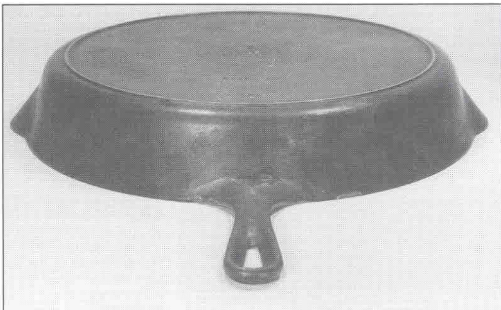
Figure 2: The skillet handle is of a different metal.
