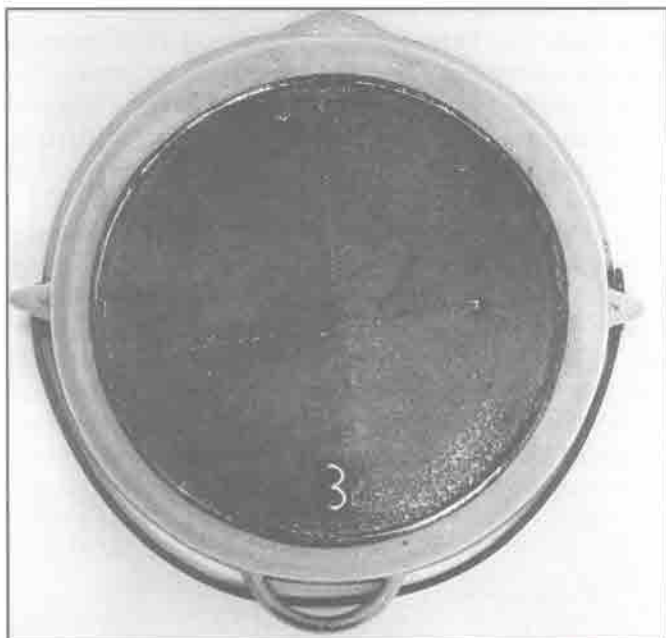
Fig. 4 Although the kettle is porcelainized, the bottom is not. Note the gate mark.
