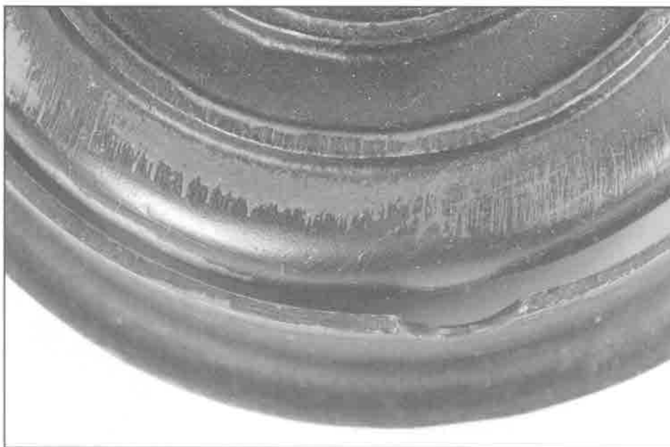
Figure 5: The outside of the paddles is very smooth. Also note the streaked wear.
