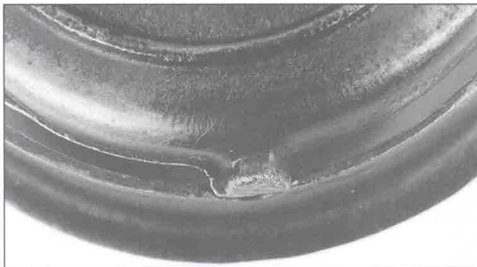
Figure 9: Stop tabs appear poorly cast and are barely long enough to touch the receiver in the base.
